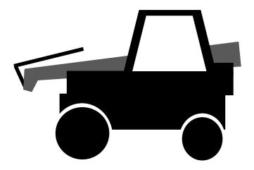
DO NOT TRAVEL ON PUBLIC ROADS WITH MACHINE LOADED because the weight of the load tends to lighten the back of the truck and could make it unstable. You may also be contravening the Road Traffic Acts (see ATB publication "Farm Vehicles on the Road").
