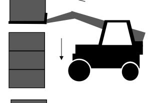
Move away from the load making sure you do not foul load on stack and stop
