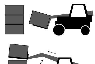
Approach stack squarely with load in travel position and stop when load is about 600mm (24in) away.
