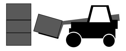
Reverse with load on, retract boom then lower boom to travel position.
