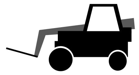
Boom fully retracted and slightly raised 300mm (12 in) off ground with or without a load and the forks tilted back.
