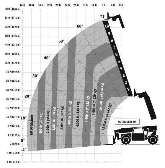
You must ensure that when lifting a load the boom is retracted to start with. Elevate the boom to the appropriate height and then extend to required height.
